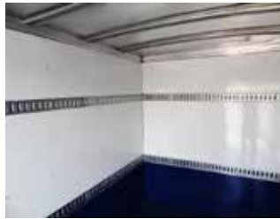
INTERIOR UPGRADES - Plywood available front & sides. Unfinished or primed & painted white. "E" track mounted over panels or recessed.
