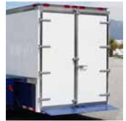
REAR DOOR - Steel welded rear door frame supports the heavy duty doors. Supported with 4 hinges & locked with strong truck door latch.
