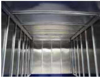
STANDARD INTERIOR - Aluminum roof & sides. Galvanized "Z" studs on 16" centers - roof bows on 24" centers. Interior completely sealed.
