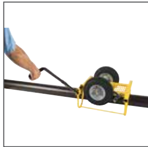
1 Use ratchet to secure Cricket to pipe
