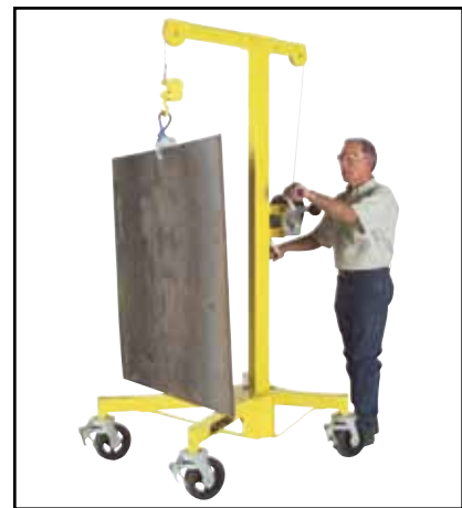
Move plate with plate lifting clamp
