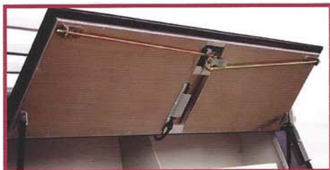
Inside Door Skin Reduces Dents From Shifting Cargo
