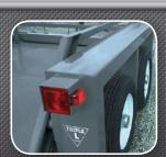
**Fenderless**No protruding fenders that are susceptible to damage.
