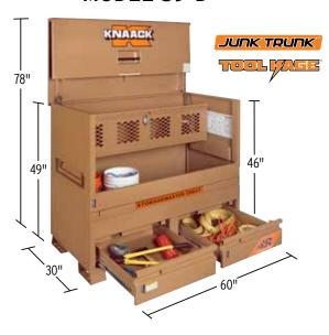
The Model 89-D STORAGEMASTER® Piano Box with Junk Trunk™ Independent Locking Drawer measures 60 in wide, 78 in tall and has a capacity of 43.8 cu ft. Ideal for mechanical trades, it is caster-ready and includes full-width shelves for organization of tools and supplies. It also features a bi-fold cover which folds completely out of the way for unrestricted access. JunkTrunk™ Quick Access Drawer locks independently for quick access to high demand tools and accessories.
